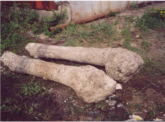
Fig. 6. Under-reamed root piles (ECE mode) in clay.
