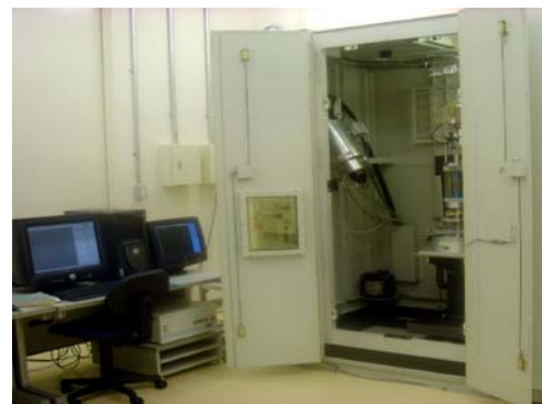
Fig. 31. Overview of micro-focus X-ray CT scanner at PARI.
