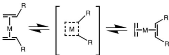
Scheme 3. The pairwise mechanism of olefin metathesis (proved incorrect)
