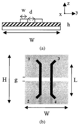
Fig. 4. System configuration: (a) cross-section, (b) top view.
