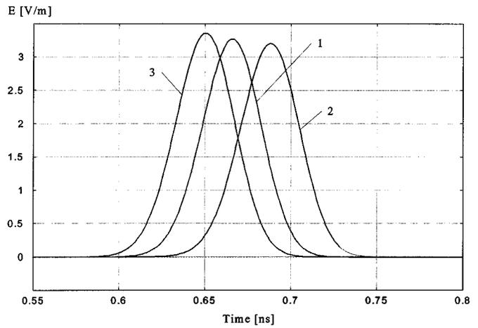
Fig. 2. Time trends of the transmitted electric field in different dielectric materials, at  $x = 9 \text{ cm}$  (origin at air-dielectric interface).
