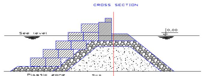
Fig.11. Cross section of the Varna's breakwater
