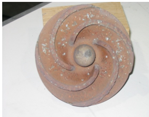
Figure 5.7. Erosion damage on the impeller surface
