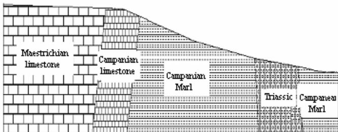
Fig. 1. Geological profile of the spillway foundation
