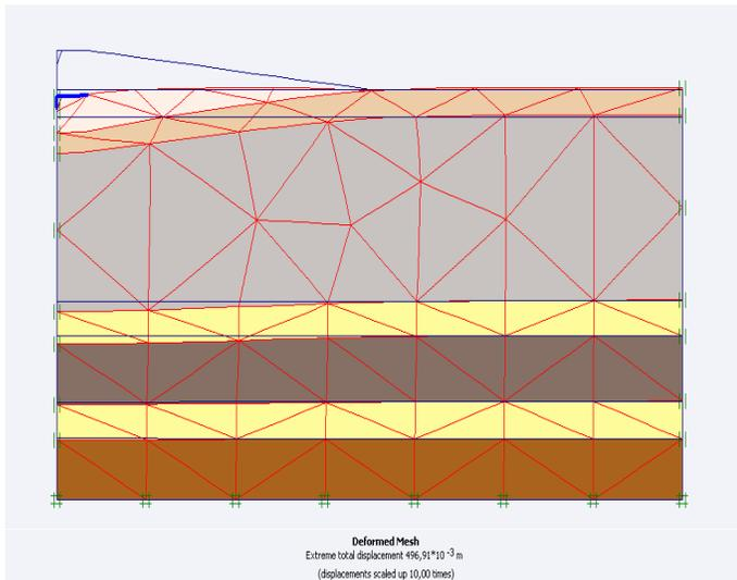
Fig.9. Vertical displacement by numerical simulation
