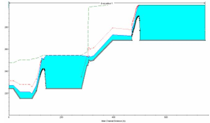
Fig. 8. Spillway water profile for a flow of 6940 m<sup>3</sup>/s
