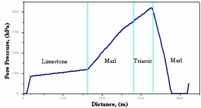
Fig. 4. Pore pressure variations along the spillway
