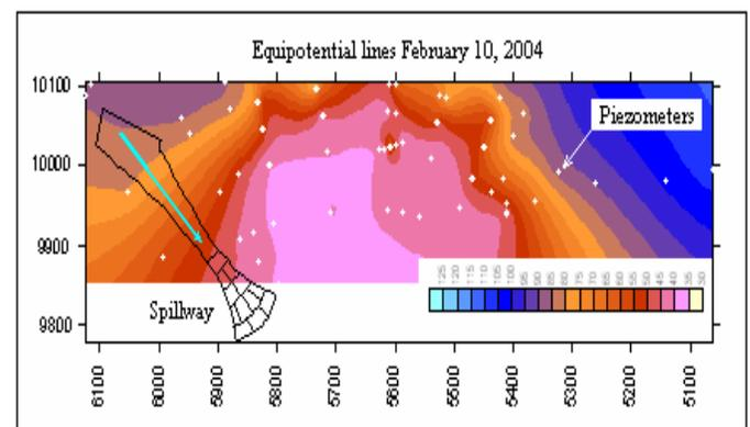
Fig. 2. Flow pattern within core dam
