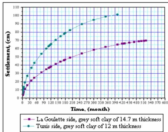
Fig.10. Settlement evolution in time: Structure KP8 + 170
