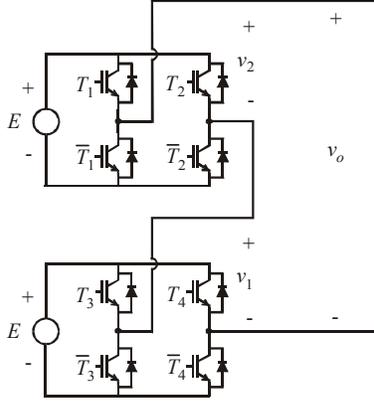
Fig. 1. Cascaded (2-cell) series H-bridge multilevel inverter with equal dc sources
