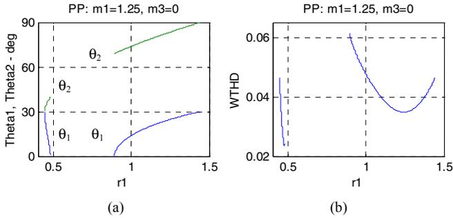
Fig. 3. (a) Step-angle solutions for varying  $\rho_1$
