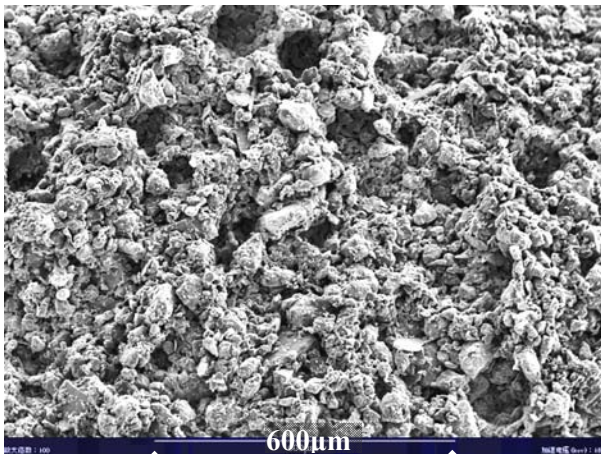
Fig.2 Microstructure of loess after liquefaction (Magnification factor: 100)
