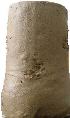
Fig.1 Loess samples after liquefaction test
