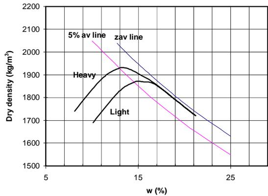
Fig. 6. Effect of compaction energy on moisture-density relationship
