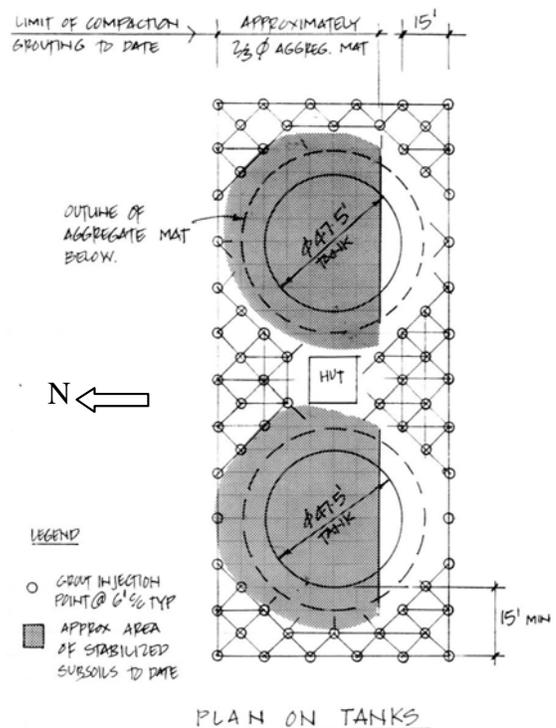
*Fig. 10. Remedial Grouting Programme*
