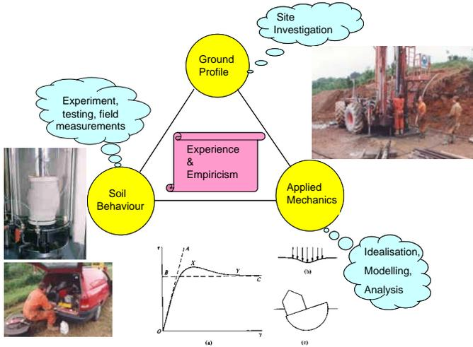
Fig. 1. Modified from Burland's soil mechanics triangle (Burland, 1989)
