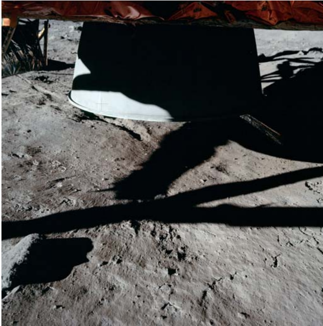
Fig. 4. Area under Apollo 12 LM engine nozzle showing how surface has been "swept clean" of loose material. The narrow trench in the upper left part of picture was dug by the soil contact probe as it dragged beneath the descending LM.
