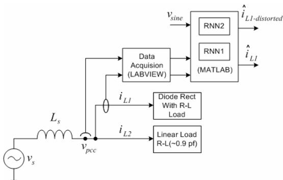
Fig. 9: Experimental setup with low voltage circuits
