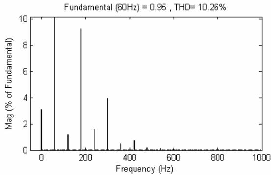
Fig. 12: FFT spectrum of  $\hat{i}_{L1-distorted}$ . THD=10.26%
