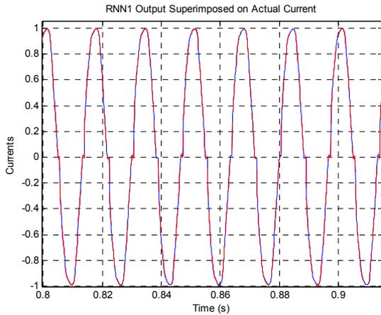
Fig. 5:  $i_1$  and  $\hat{i}_1$  superimposed
