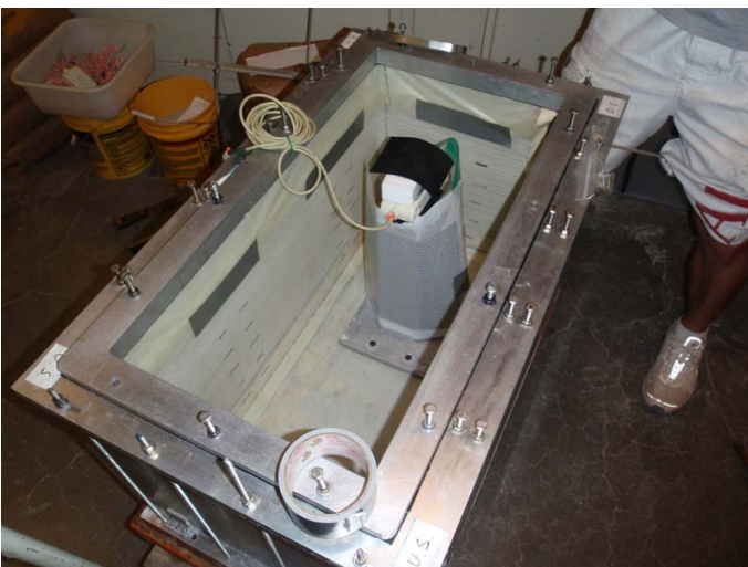
Fig. 15 Instrumented caisson installed in the laminar box for Experiment I-A2. Instrument handle is placed atop the caisson.
