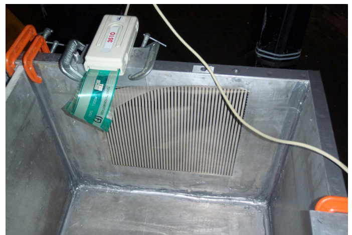
Fig. 10 Laminated tactile pressure sensor installed in rigid, split box.
