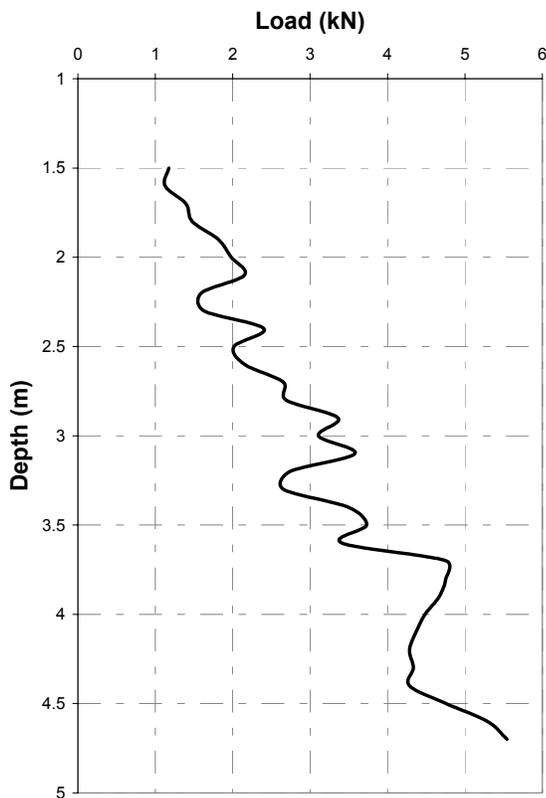
Figure 3: Load during installation
