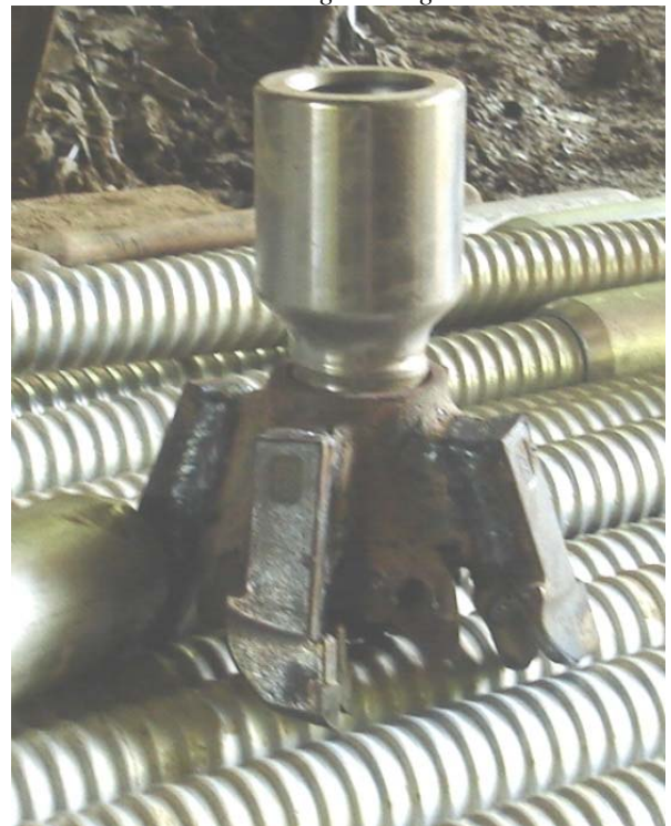
Fig. 4. Drilling of test hollow core bar micropile through casing.
