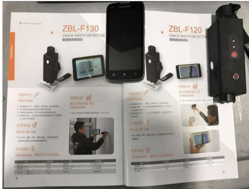
Fig. 5 – Crack width detector.
