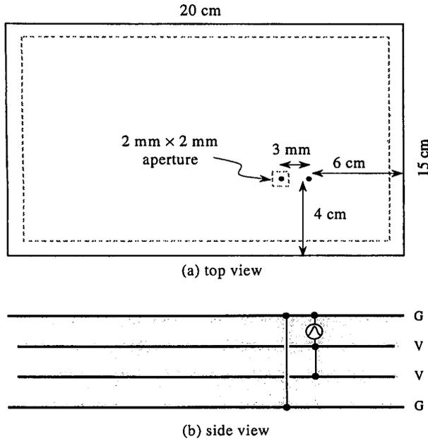
Figure 3. Schematic of the GND-VCC-VCC-GND power bus stack for the FDTD modeling.
