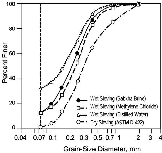
Fig. 4. Summary of various sieve analysis test results
