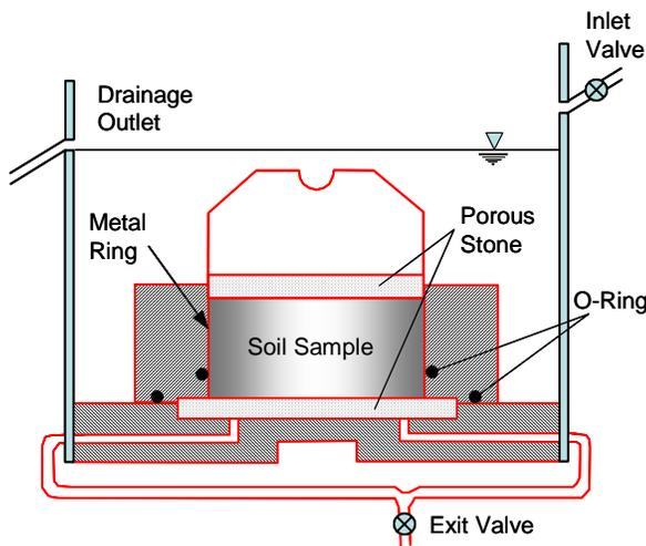
Fig. 3. Schematic diagram for the modified oedometer
