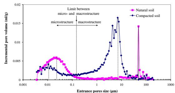
Fig. 1 - Pore size density function evaluated from MIP results
