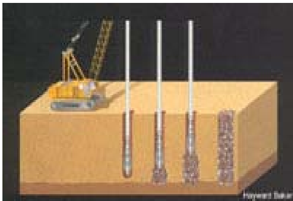
Plate-1: Stone Column Procedures
