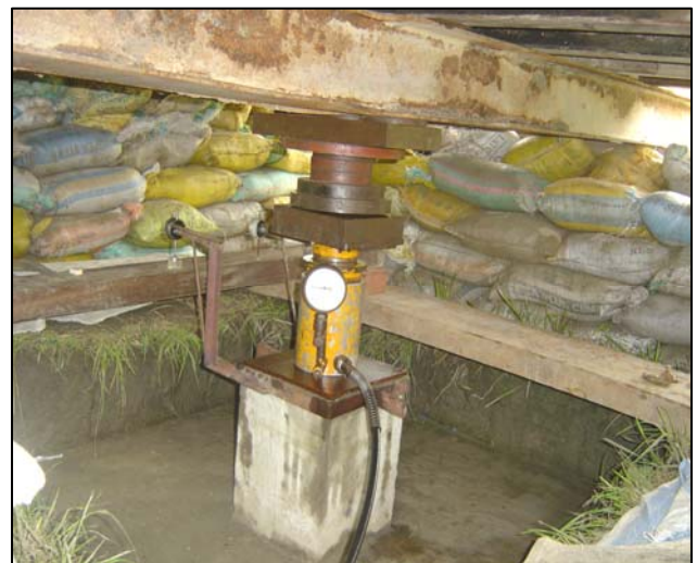
Fig. 6. Full scale footing load test arrangement
