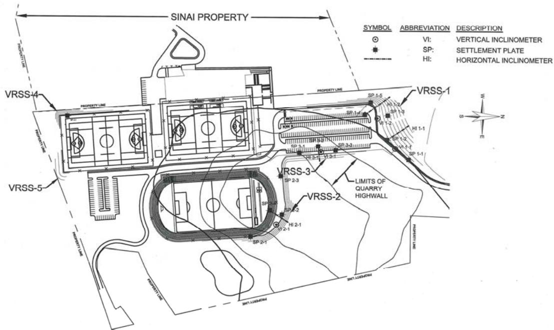
Fig. 8. Instrumentation Locations
