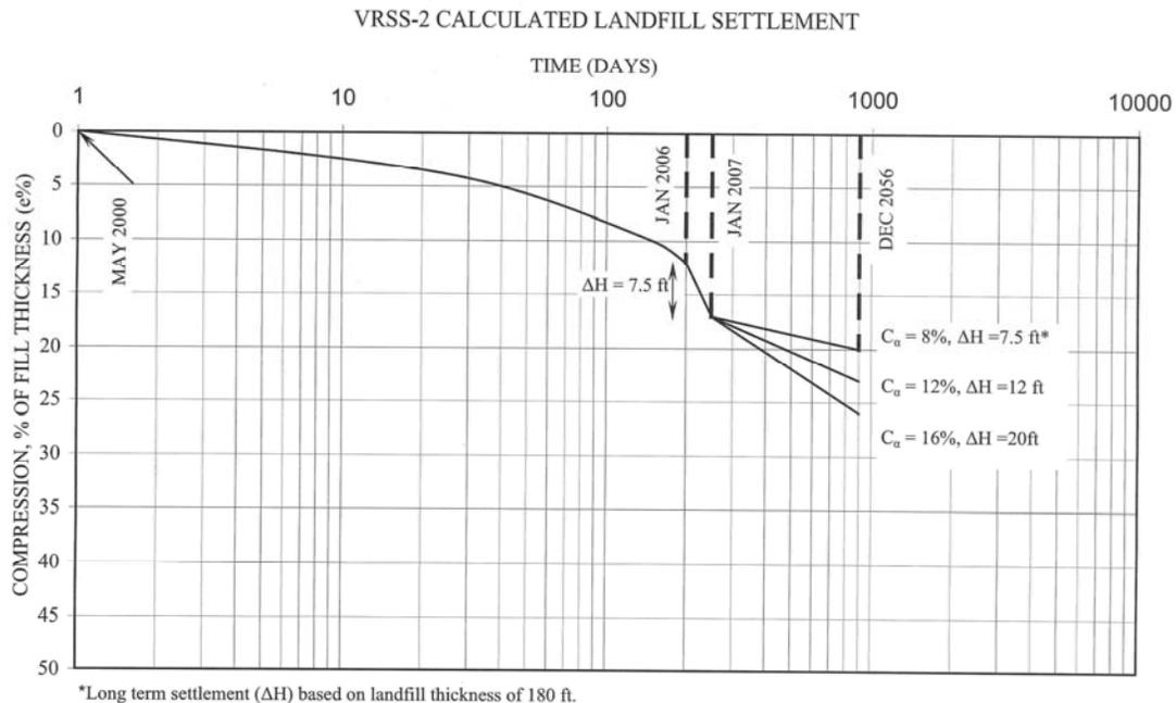
Fig. 5. Plot of Estimated Settlement during Design Life
