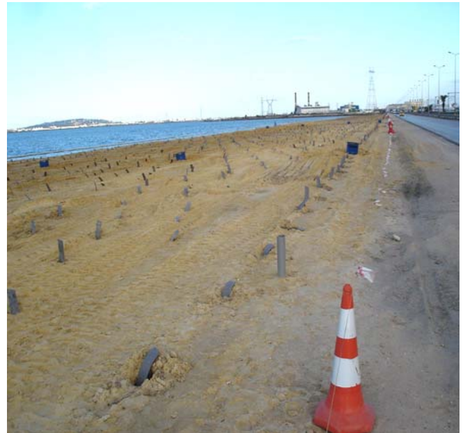
Fig. 17. Locations of settlement recorders in PVD improved soil.
