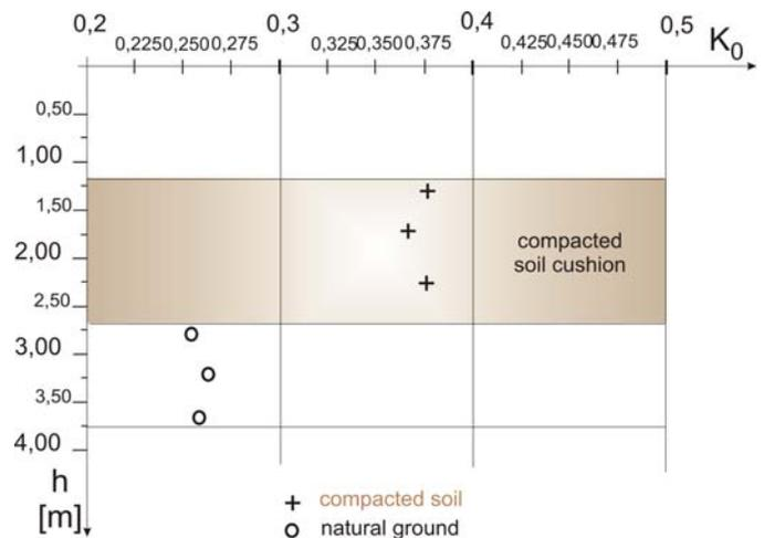
Fig.2. The bonding coefficient  $K_0$  variation over depth
