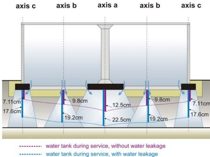
Fig.16. The advance of the water front and the settlement diagram according to the 3<sup>rd</sup> hypothesis
