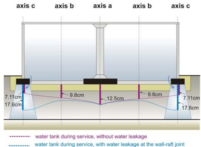
Fig.15. The advance of the water front and the settlement diagram according to the 2<sup>nd</sup> hypothesis
