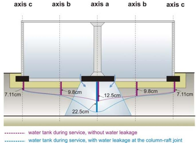
Fig.14. The advance of the water front and the corresponding settlement diagram according to the 1<sup>st</sup> hypothesis
