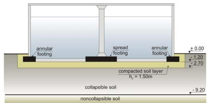
Fig.1. Current vertical section of the water tank
