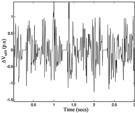
Figure 10. PRBS signal applied to the excitation system of generator G4,  $\Delta V_{ref4}$ .
