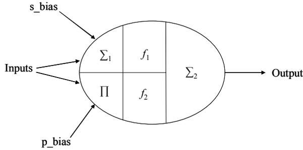
Figure 4. Dual function neuron model.
