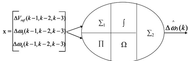
Figure 6. DFN structure of WAM estimating speed deviation of G3.
