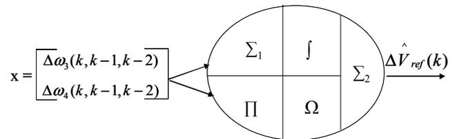
Figure 8. DFN structure for nonlinear controller.
