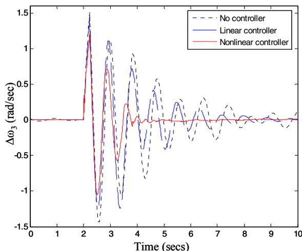
Figure. 16. Speed deviation of generator G3 for line 4-6 outage and a three phase short circuit fault of 200ms halfway between 7 and 8.
