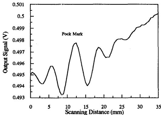
Fig. 3 Detected signal for a pock mark at a frequency of 31.5 GHz, and at 3 mm standoff distance (without a horn antenna) [1].
