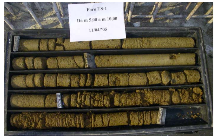
Fig.5. Typical tuff samples recovered by coring
