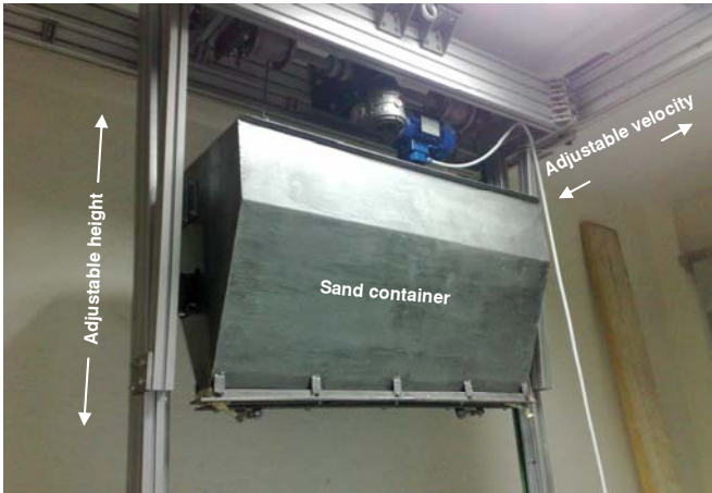
Fig. 5. Sand raining system used for model preparation.
