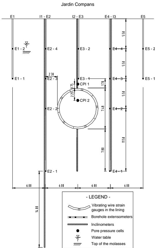
Fig. 3. Compans monitoring section S23: transverse view
