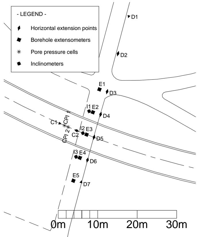
Fig. 4. Compans monitoring section S23: plane view
