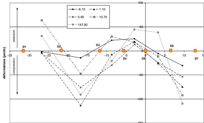
Fig. 11. Ground surface horizontal extension – transverse profile
