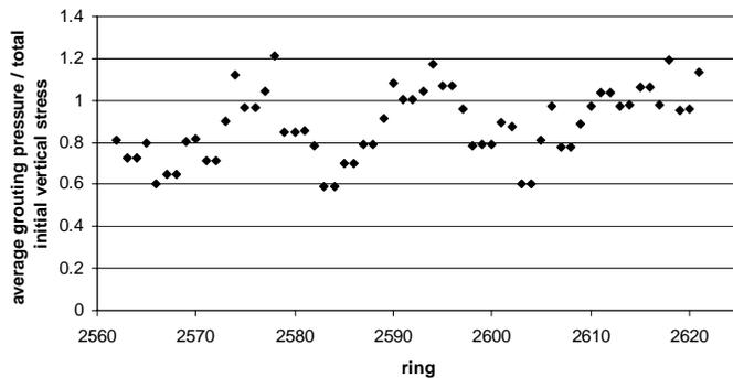
Fig. 21. TBM grouting pressure
