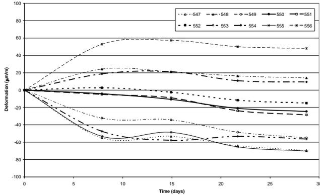
Fig. 18. Induced strains in the concrete lining
