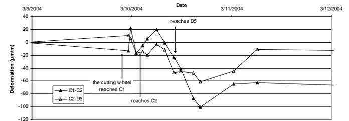
Fig. 13. Ground surface horizontal extension – longitudinal profile
