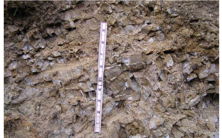
Figure 3: View of the siltstone rock mass in a test pit at shallow depths (scale is 1 ft=30.5 cm)
