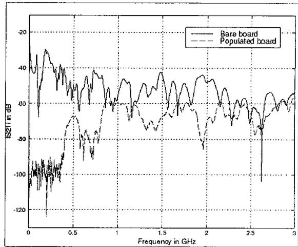
Figure 8: Measured S21 on bare and populated boards
