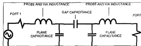
Figure 2: Circuit model of simple power island structure
