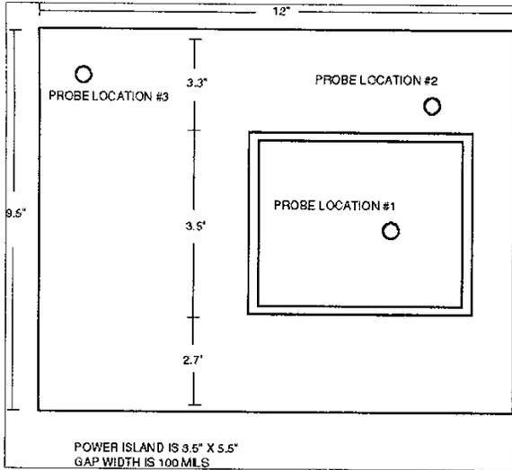
Figure 6: Power island location in a PC motherboard
