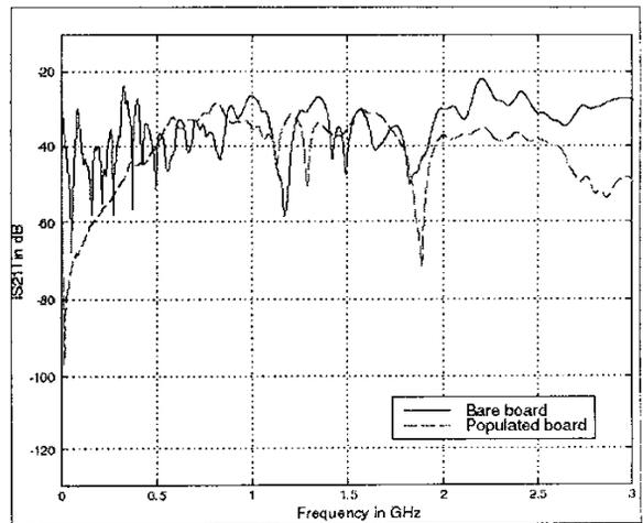
Figure 10: Measured S21 between distant probe locations
