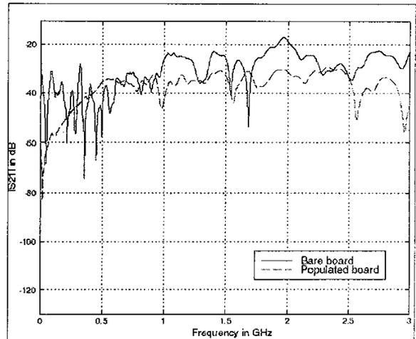
Figure 9: Measured S21 between probes in close proximity
