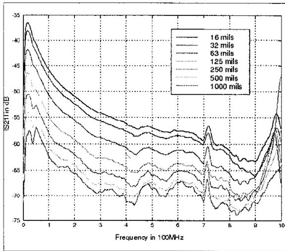
Figure 3: Effect of gap width on coupling
