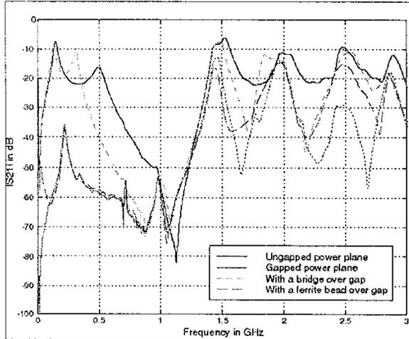
Figure 4: Effect of bridge on power island coupling
