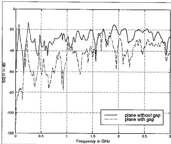
Figure 7: Measured S21 with and without power island
