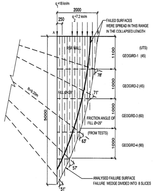
Fig.6. Section of RSR Wall showing Critical Surface Analysed
