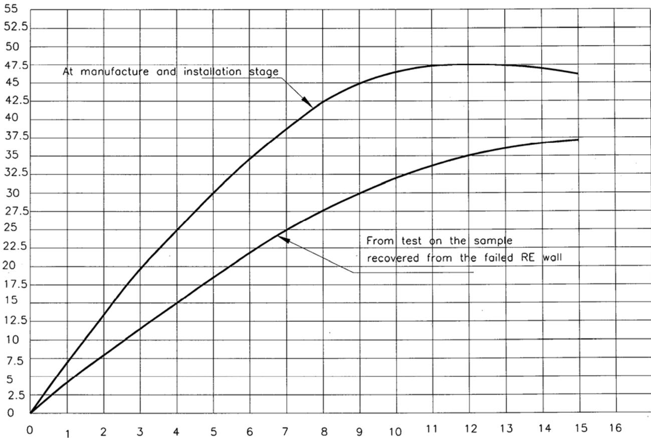
Fig.5. Stress-Strain Relationship of the Geogrid (UTS 45 kN/m) – at Installation and at Failure
