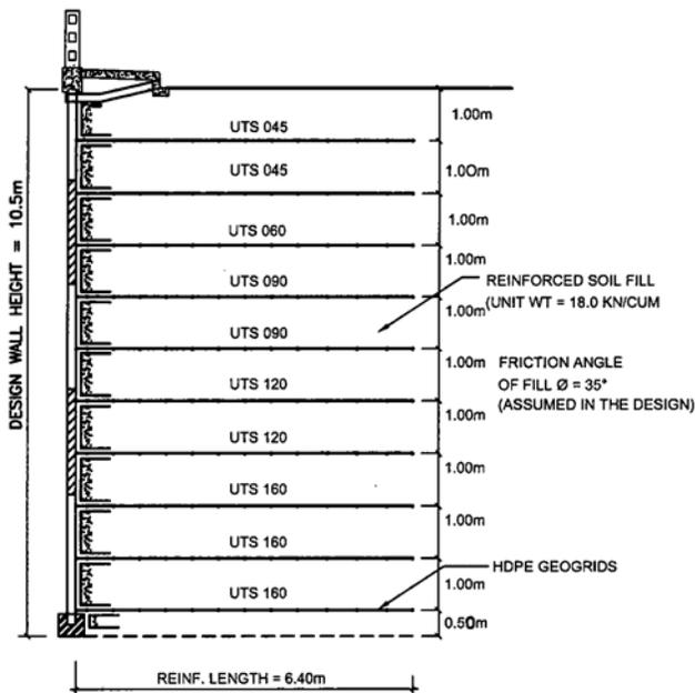
Fig.4. Cross Section of RSR wall as Built
