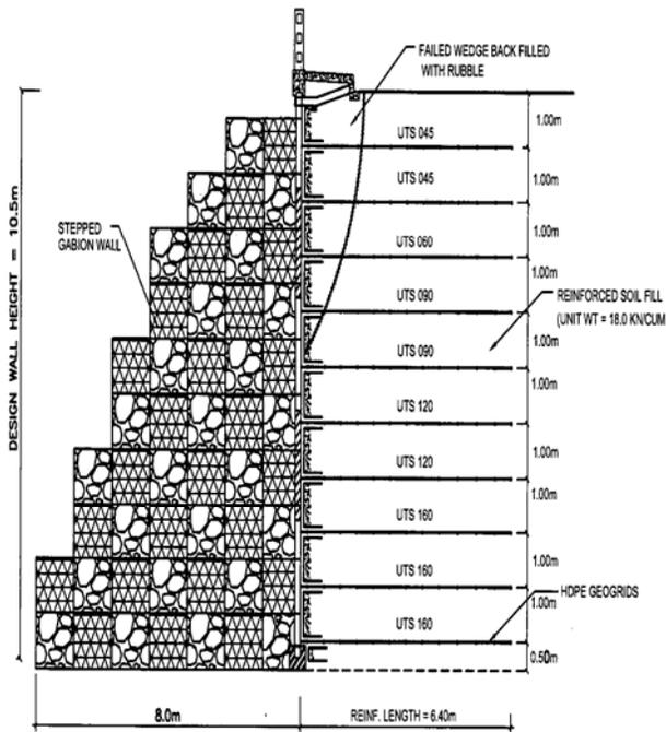
Fig. 7. Stepped Gabion Wall Built to Protect the Failed Section
