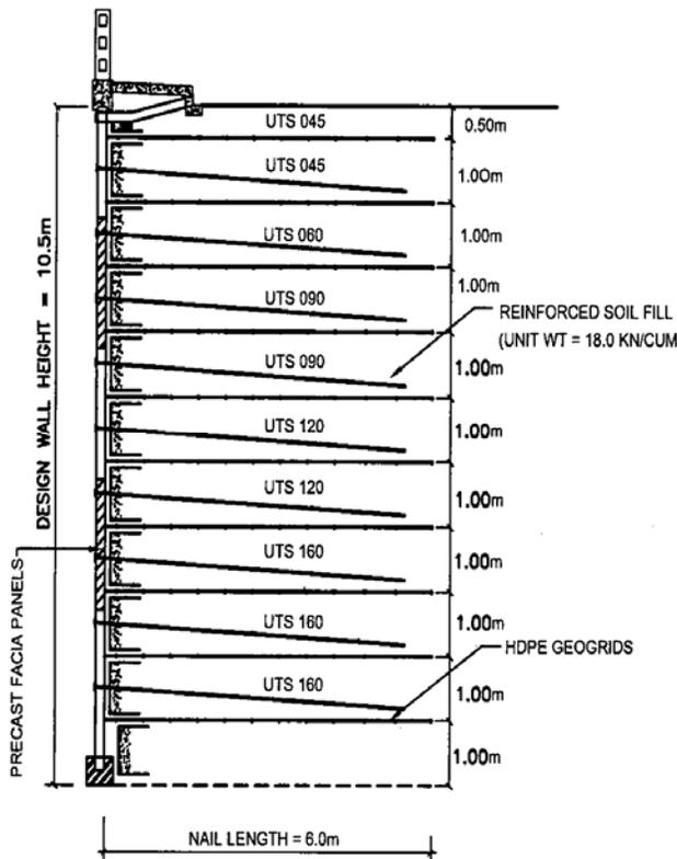
Fig.8. Cross Section of RSR Wall with Steel Nails
