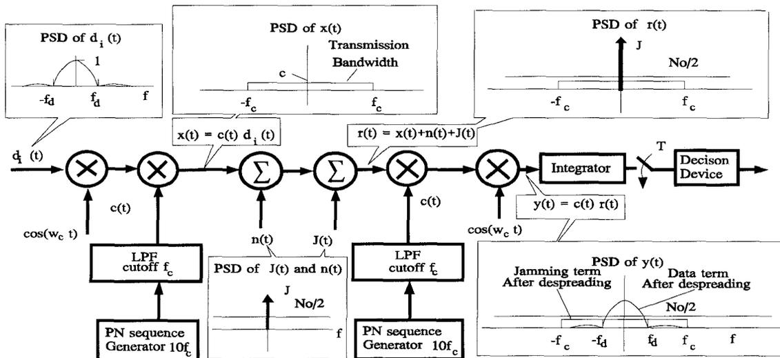
Figure 2 BLWGN DS-SS system block diagram.
