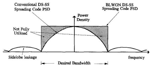
**Figure 1** Power spectra of conventional and BLWGN codes.
