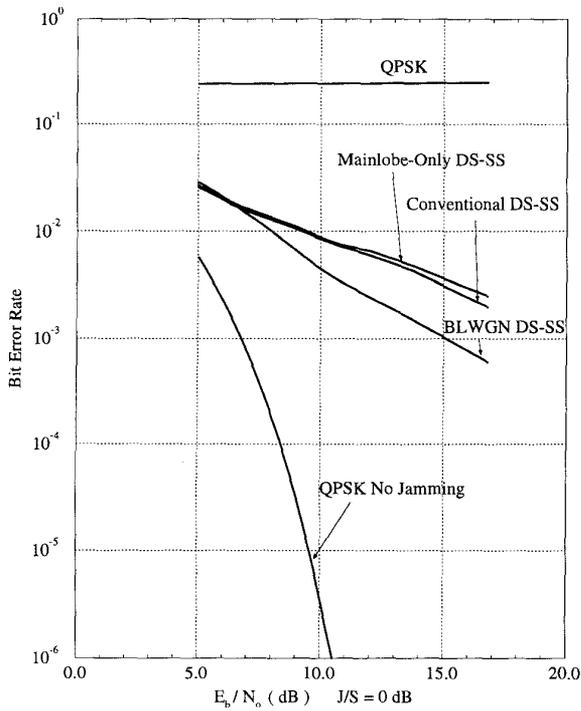
**Figure 4** Performance in tone jamming. (Jamming at carrier frequency).
