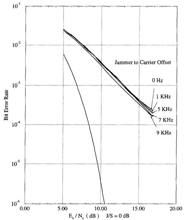
**Figure 6** Performance of BLWGN SS system in tone jamming.
