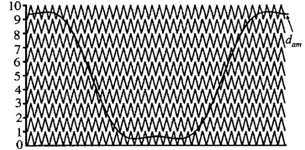
a) modified duty cycle and triangle waveforms
