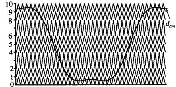
a) modified duty cycle and triangle waveforms
