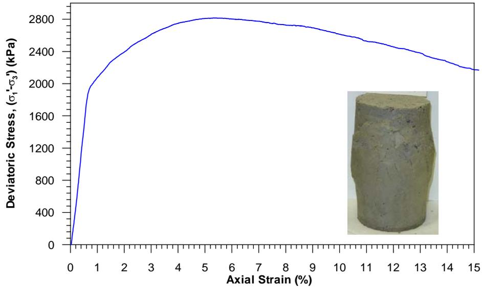
Figure 9 – Typical CU Triaxial Stress-Strain Test Results of Plastic Concrete Trial Mixes
