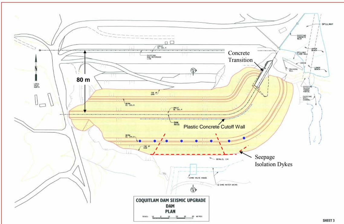
Figure 3 – New Downstream Earth Core Rockfill Dam – Plan
