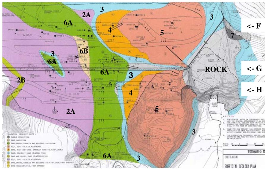
Figure 5 – Surficial Geological Units for Coquitlam Dam Site
