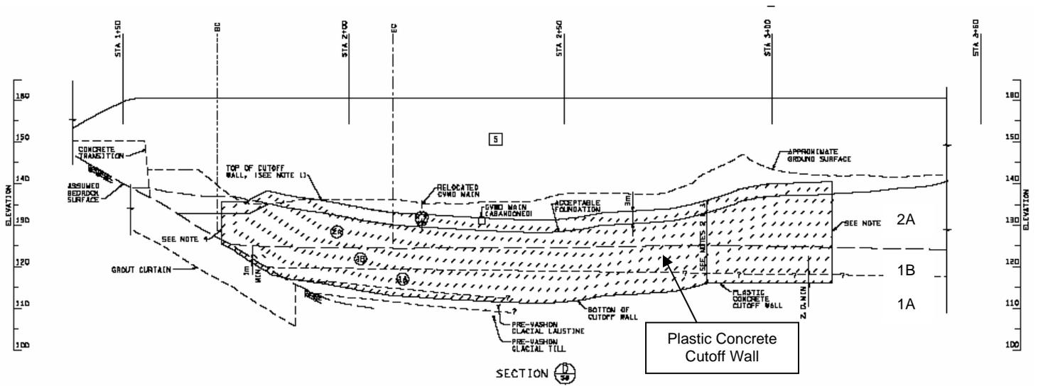
Figure 7 – Longitudinal Section of the Cutoff Wall (Looking Downstream)
