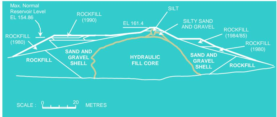
Figure 2 – Cross Section of Existing Coquitlam Dam
