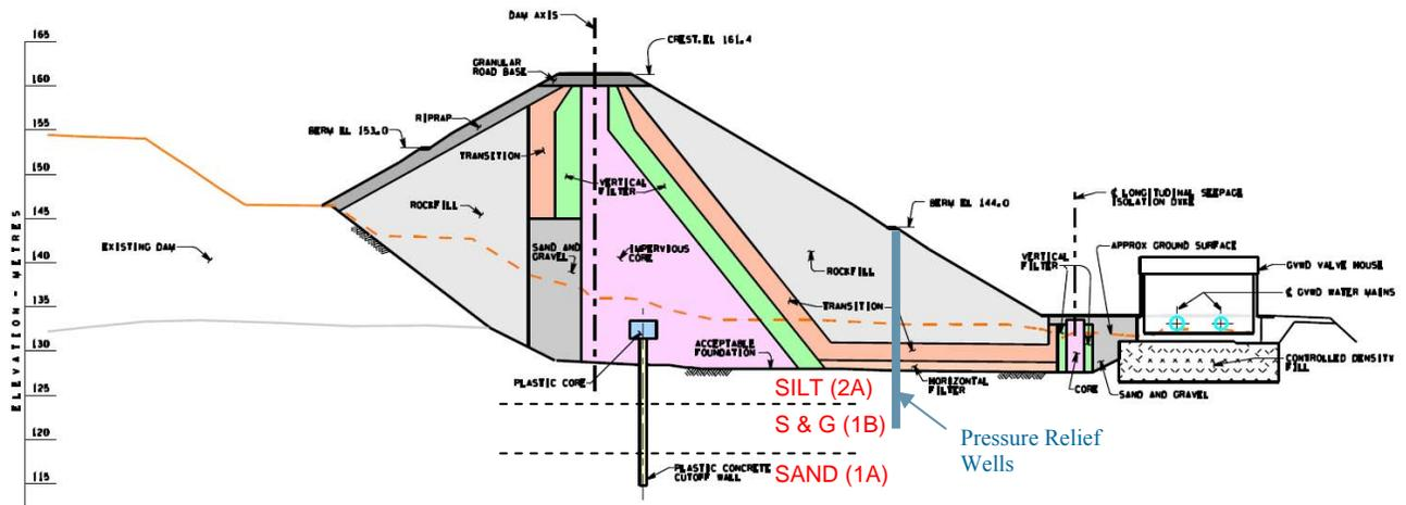
Figure 4 – Typical Section of New Downstream Rockfill Dam
