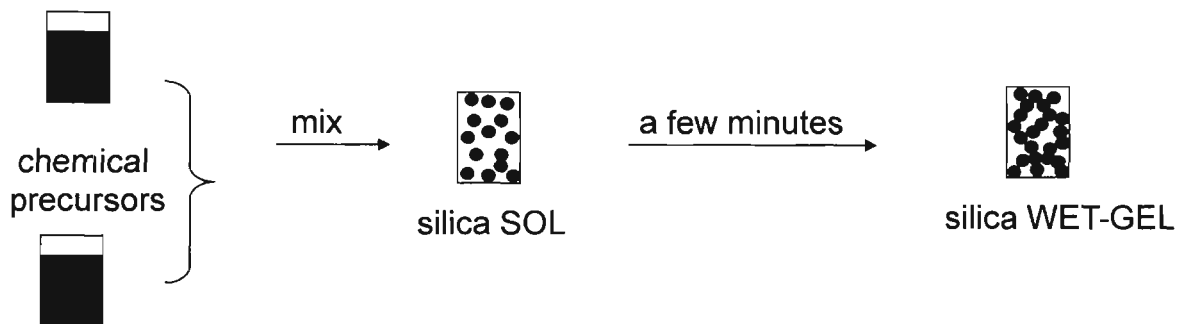
Figure 1.1 Preparation of a silica gel by the sol-gel process: (A) Chemically. (B) Experimentally.
