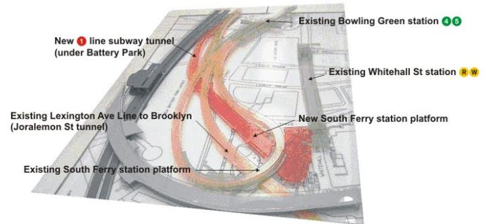
*Fig. 2. Project Location – New Tunnel Configuration*
