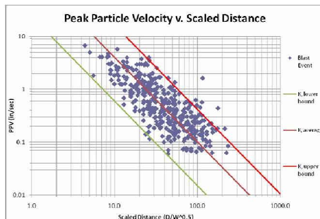
Fig. 11. Scaled distance log-log plot of data
