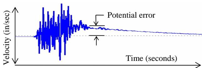
Fig. 5. Waveform, example of faulty seismograph reading
