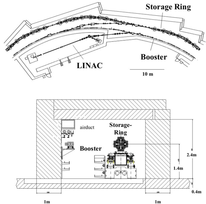
Fig. 1. Facility layout and section through the booster and storage ring tunnel
