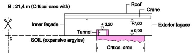
Fig. 3. Ground plan and section of main building at ALBA
