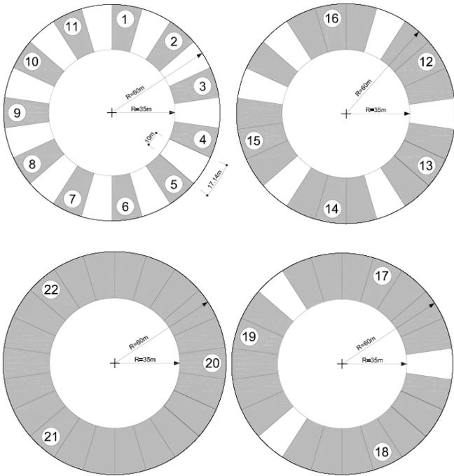
Fig. 10: Sequence of pouring the single elements of the test area slab
