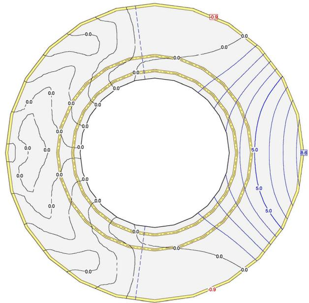
*Fig. 4. Example of deformation pattern of a stiff plate directly founded on the soil*
