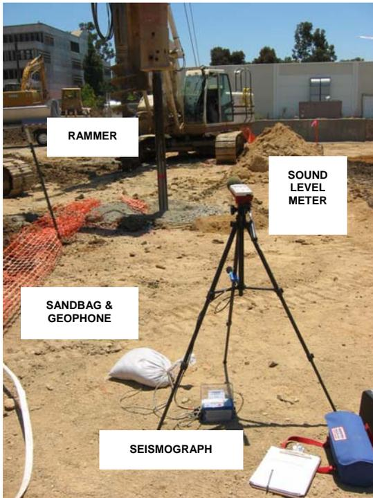
Fig. 4 Photograph showing typical instrumentation set-up.
