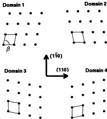
FIG. 2. The four real-space orientational domains of the vortex lattice formed for magnetic fields applied parallel or nearly parallel to the  $c$  axis. An appropriate superposition of the diffraction patterns from these domains explains the data of Fig. 1. The top row of that figure is taken under conditions in which only two of the domains are populated (1 and 2 or 3 and 4). In the bottom row all four domains are populated.
