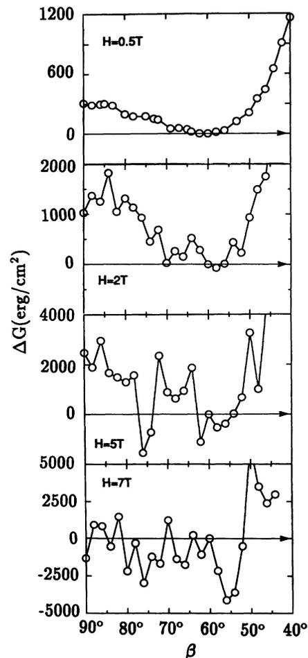
FIG. 3. Numerically computed Gibbs free energy densities of vortex lattices with centered rectangular symmetry, as a function of the angle  $\beta$  between primitive vectors (Fig. 2), relative to the triangular lattice ( $\beta = 60^\circ$ ). The calculations are based on the London model with  $\lambda = 1500\text{\AA}$  and  $\xi = 16\text{\AA}$ . The numerical errors are much smaller than the symbol size.
