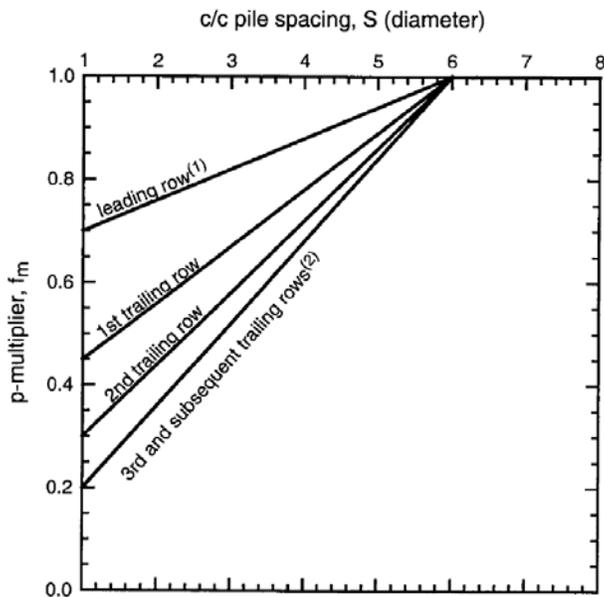
Fig. 3. P-multiplier design curve (Mokwa and Ducan 2001)
