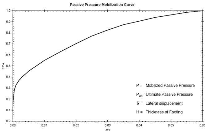
Fig 1. Passive Pressure Mobilization Curve (FEMA, 2000)
