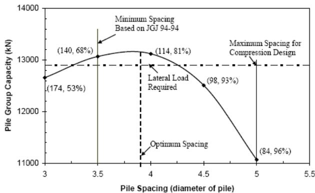
Fig. 5. Pile group lateral capacity versus pile spacing
