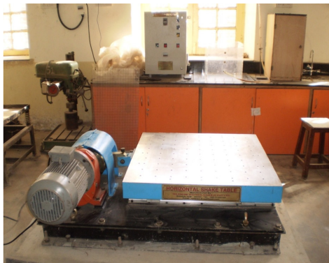
Photograph 1. Shake Table Apparatus
