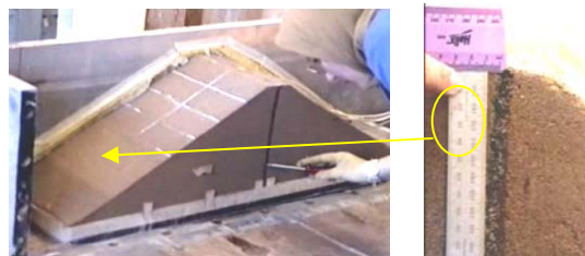
Fig.13. Displacement of asphalt core in centrifuge model test
