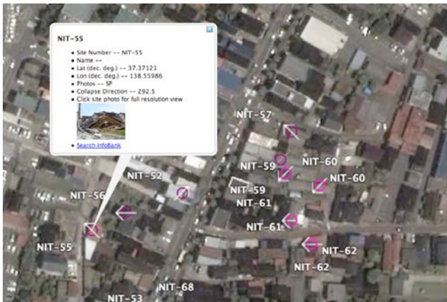
Figure 6. Detail of house collapse at site NIT-55 with collapse vectors indicating direction of fall.
