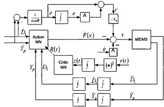
Fig. 4. Structure of the NN controller.
