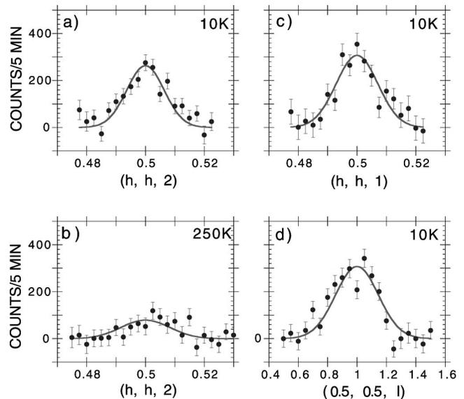
FIG. 1. (a) Scan along  $h, h$ , through the  $(0.5, 0.5, 2)$  reflection at 10 K. (b) shows the same scan at 250 K. (c) Scan along  $h, h$ , for the  $(0.5, 0.5, 1)$  reflection at 10 K. (d) Scan along  $l$  for the  $(0.5, 0.5, 1)$  reflection at 10 K. The lines are gaussian fits to the data. A background determined from the scans at  $(0.5, 0.5, 0)$  has been subtracted from the data. The counting time was 5 min per point with multiple scans averaged to obtain the counting errors shown.
