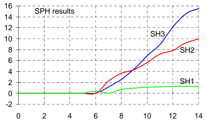
Fig. 10. Comparison of failure horizontal displacement between the experiment and the SPH simulation.
