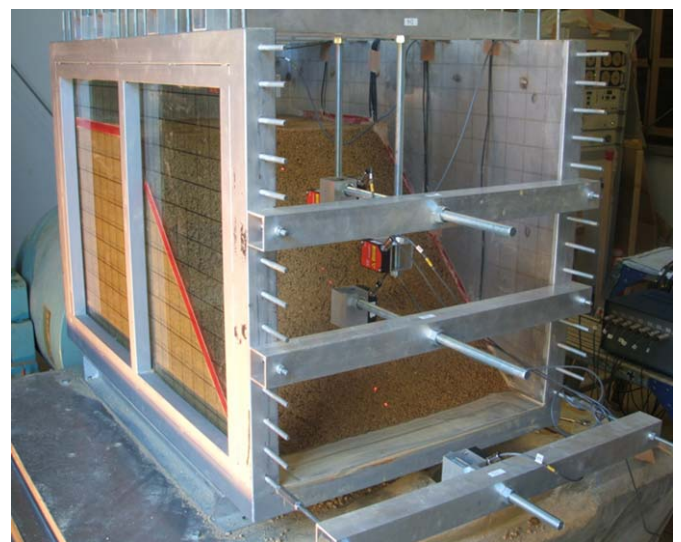
Fig. 4. Overview of slope model after construction.
