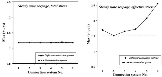
Fig. 8. Comparison of the ratio of major principal stress to minor principal stress in different connection zones at the two phases of the end of construction and steady state seepage
