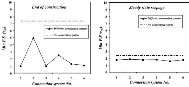
Fig. 12. Comparison of factors of safety against shear stress for different connections at the two phases of the end of construction and the steady state seepage
