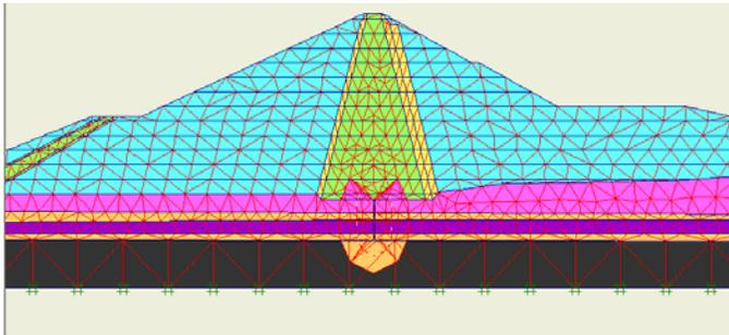
Fig. 3. Finite element mesh generated for the dam
