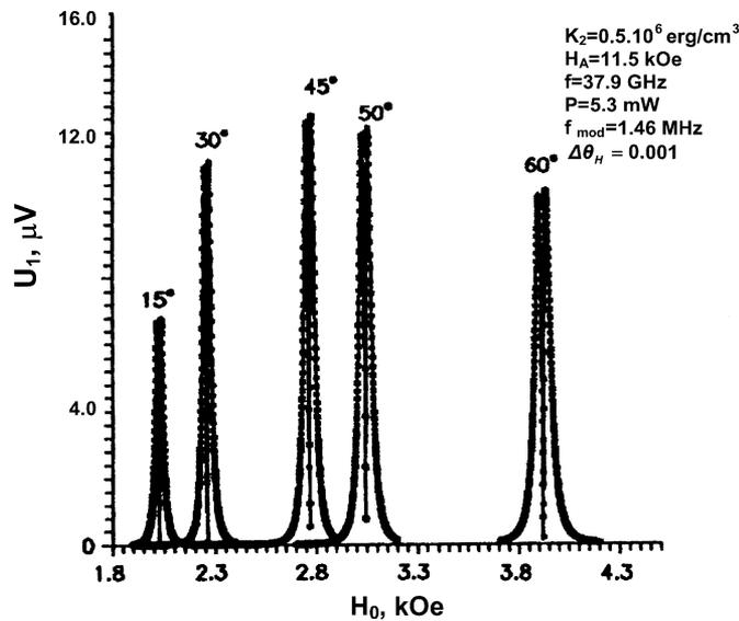
Fig. 9. The calculated first harmonic of modulation frequency at different angles of orientation of ferrite  $\theta_H$ .
