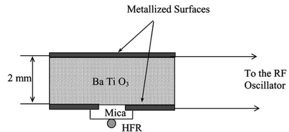
Fig. 6. Piezoceramic-HFR structure.
