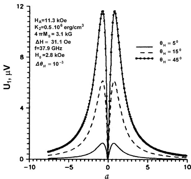
Fig. 10. The first harmonic of modulation versus the relative detuning from resonance at different angles of orientation.
