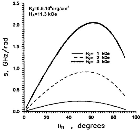
Fig. 2. Dependence of speed of resonance frequency variation upon angle of HFR orientation.
