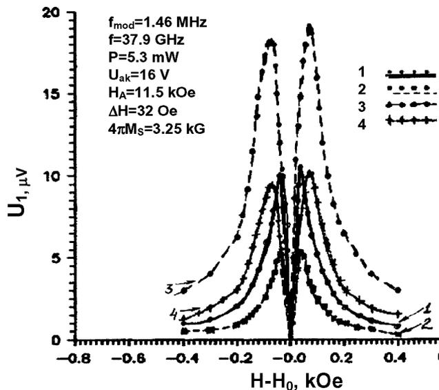
Fig. 13. The first harmonic of modulation frequency at different angles of orientation of ferrite: 1:  $\theta_H = 45^\circ$  without capsule; 2:  $\theta_H = 15^\circ$  without capsule; 3:  $\theta_H = 45^\circ$  with capsule; 4:  $\theta_H = 15^\circ$  with capsule.
