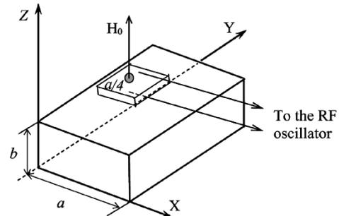
Fig. 5. Waveguide with HFR and piezoceramic slab inside.
