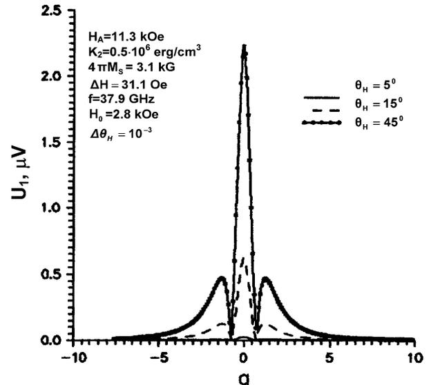
Fig. 11. The second harmonic of modulation versus the relative detuning from resonance at different angles of orientation.
