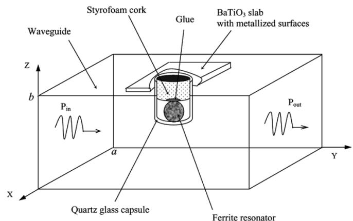
Fig. 12. Structure HFR-PES with a quartz capsule in the waveguide.
