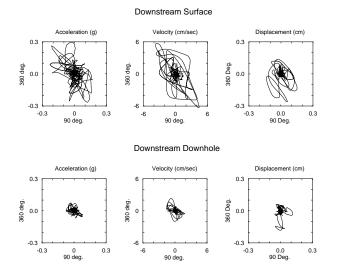
Fig. 6. Horizontal particle acceleration, velocity and displacement at the downstream surface and downhole instruments during the Yucaipa earthquake.
