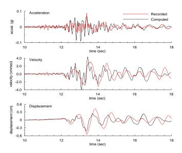
Fig. 10. Calculated and recorded time histories at the crest downhole instrument for the Yucaipa earthquake – 3-D analysis
