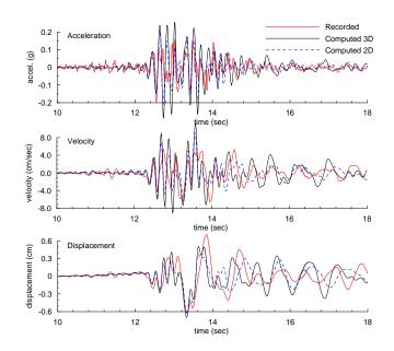
Fig. 17. Comparison of N-S motions calculated at the crest surface from 2-D and 3-D analyses with recorded motions – Yucaipa earthquake
