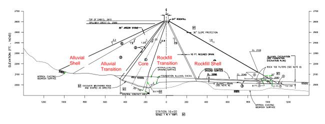
Fig. 2. Maximum cross section of Seven Oaks Dam.
