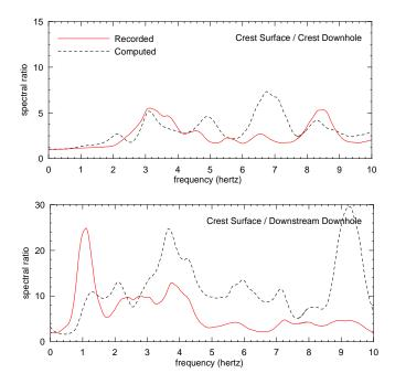
Fig. 16. Calculated and recorded N-S acceleration Fourier spectral ratios for the Big Bear Lake earthquake – 3-D analysis
