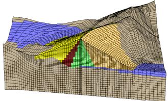
Fig. 8. Three-dimensional finite element mesh of dam
