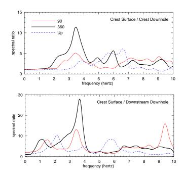
Fig. 7. Fourier spectral ratios between selected acceleration records from the Yucaipa earthquake.
