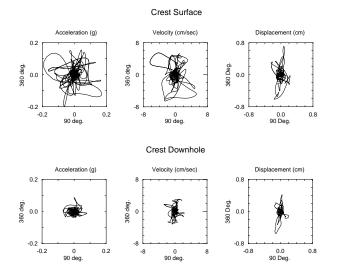
Fig. 5. Horizontal particle acceleration, velocity and displacement at the crest surface and downhole instruments during the Yucaipa earthquake.
